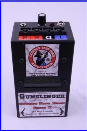
The top of the timer is where all connections are made from the Controller and to other timers hooked in series, the target, and the audience display. It is also where the power supply and elimination cord are connected. It also has the sensitivity adjustment knob.
