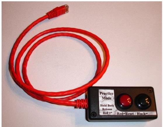
immediately to "Reset and Ready to Start". By depressing the "RED" Reset Button it immediately erases all times on the timer and the Audience Display and is instantly ready to start. Note: Once the reset button is pressed you may not recall times that have been erased.
